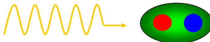
$$\begin{aligned}\vec{p} &= \alpha \vec{E} \\ \vec{\mu} &= \beta \vec{H}\end{aligned}$$
